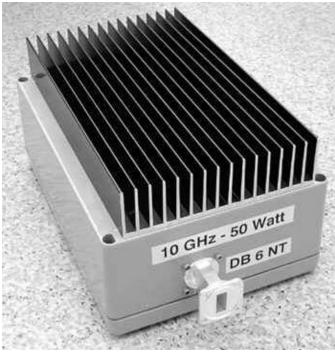
This x-band transverter was built for the 60 ft. dish at the AMSAT DL Bochum site to be used for EME and Tropo. The purpose is to get ready for the Mars mission and other deep space endeavors. The amplifier puts out 50 Watts on 10 GHz. The receiver has a noise figure of .65dB and the 144 Mhz input power required is 3 W
