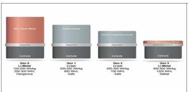
SolidEnergy Systems' battery (located at far right) is twice as energy-dense as the lithium ion batteries used in consumer electronics.
