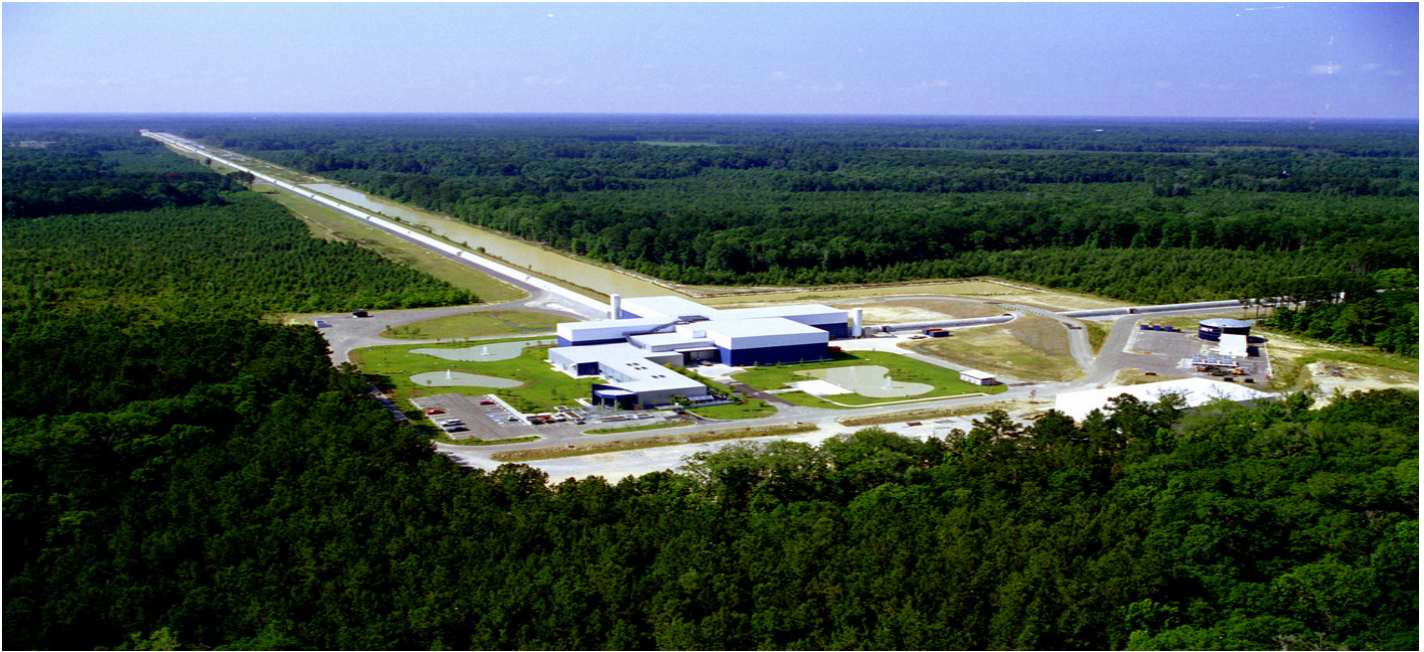
Aerial photo of LIGO Livingston, Louisiana, showing all of one 4 km long arm and part of the other (off to the right). The visible arms are concrete structures that protect the vacuum tubes from the elements. (Credit: Caltech/MIT/LIGO Lab)
