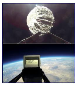
The reading on the LCD screen shows a dose rate of 3.7 uSv/hour, more than 20 times higher than radiation levels at the launch site. Another independent sensor was contained inside a thermally insulated capsule. Working together, the two sensors measured a complete profile of ionizing radiation from 2.8 km to 27 km above Earth's surface.
