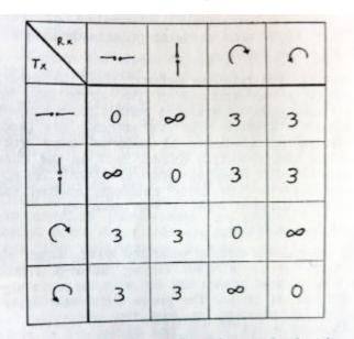
Fig. 7 — Interaction of various polarizations (extra attenuation in dB).
