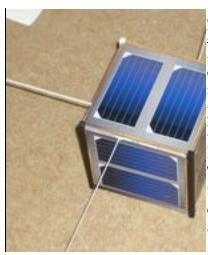
Scheduled to be among the other Amateur Radio-payload carrying satellites is <u>FUNcube-1</u>, a 1U CubeSat that is a collaboration between AMSAT-UK and AMSAT-NL. It will carry an "educational beacon" (1200 baud BPK -- daytime operation) and a 20 kHz wide U/V inverting SSB/CW transponder running 300 mW PEP (nighttime operation). A project begun in 2009, FUNcube-1 will provide a signal *directly* to schools, with the "target audience" students at the primary and secondary levels.
