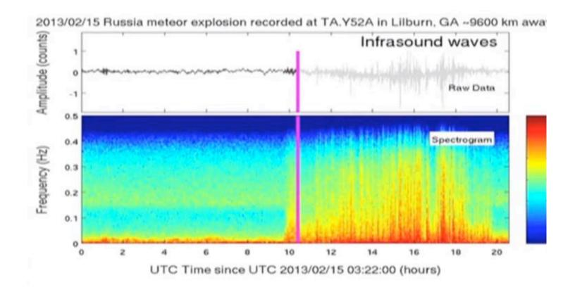
Infrasound signals associated with the Russian meteor impact on February 15, 2013, recorded nearly 9,600 km away in Lilburn, Georgia. The sound took about 10 hours to travel from Russia to Georgia. (Credit: The seismic data is distributed by the IRIS DMC, TA/USArray network/Image from video courtesy of Georgia Institute of Technology)
