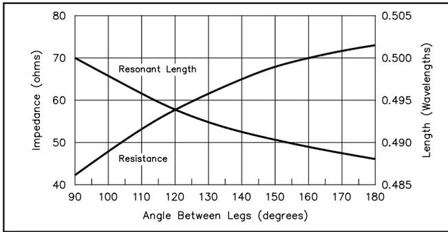
**Fig 8-21—Radiation resistance (resistance at resonance) of the inverted-V dipole antenna in free space as a function of the angle between the legs of the dipole (apex angle). Also shown is the physical length (based on the free-space wavelength) for which resonance occurs.**
