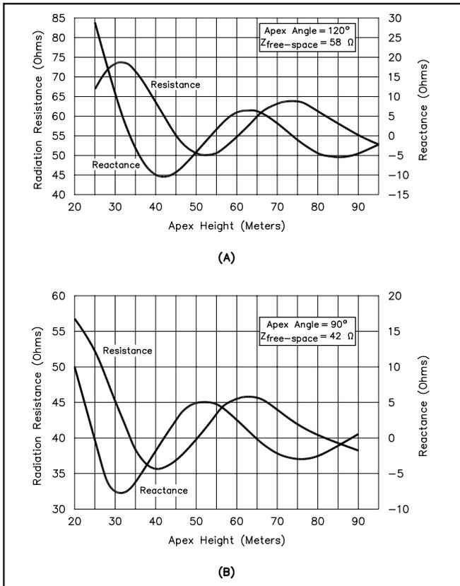
**Fig 8-22—Impedance (feed-point resistance and reactance) of inverted-V dipoles as a function of height above ground. Analysis frequency is 3.75 MHz, with a 2-mm OD wire (AWG #12). Resistances at resonance are: 120° apex angle, 58 Ω; 90° apex angle, 42 Ω. NEC-2 was used for these calculations, since MININEC is unreliable for impedance at low heights.**
