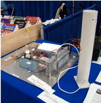
The 70cm/in 13cm/out Linear Transponder the white cylinder contains a Yagi pointed straight up
